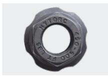
GRIP-TIGHT™ Nuts have M22X1.5 threads, 33mm hex, 27mm height and a 46mm washer diameter. The two-piece GRIP-TIGHT™ Nuts comply with technical requirements of SAE J1965. Cross Reference PN's: 39773, 39874, 39702, M3979, 39691, 39949, 201.3013, 13-3057, E-9020, W-525, R009020, 511034, KB9020,WA075037, 20857204, 1649492C1, E6HZ-1120-A, MF110343, and MF111026.
